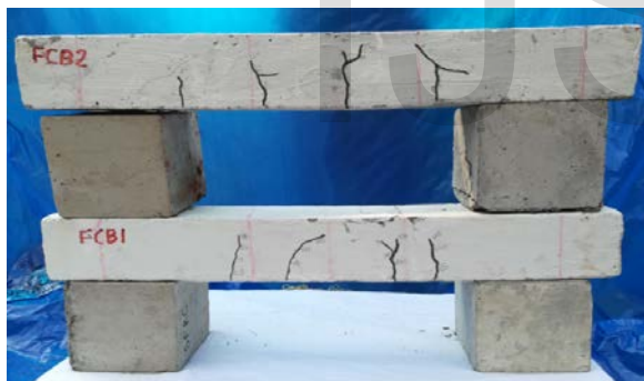
Fig.6 Failure pattern of flexural control beams
