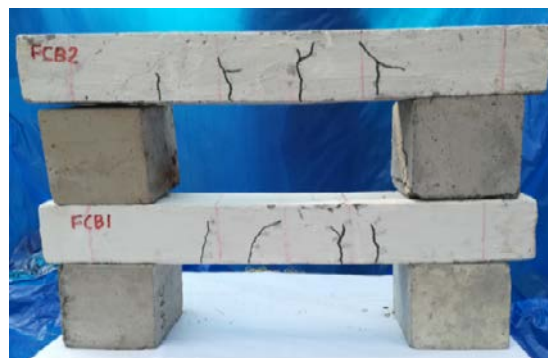
(a) Beams after experimental testing
